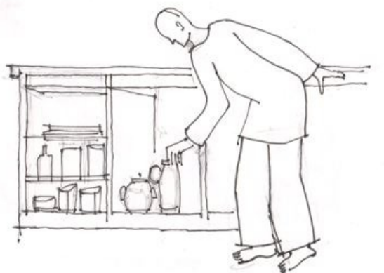
AVOID LOW-DOWN STORAGE PLACES IN KITCHENS
